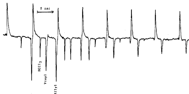
Figure 2.—Repeated scans of the CIDNP spectrum, taken at 19.3 MHz, during the thermolysis of trichloroacetyl peroxide in carbon tetrachloride solution of TME. The strong absorption peak is TME. Sweeps were from low to high field with flyback from 1 to 8 ppm.
